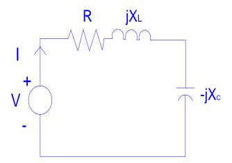
Figure 1. Series resonance circuit example.
