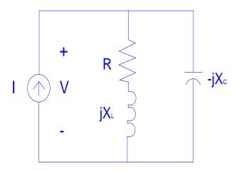
Figure 5. Common parallel resonant circuit
