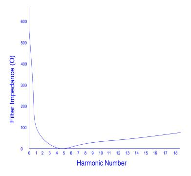
Figure 22. Frequency response of single-tuned filter
