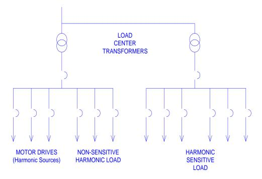
Figure 25. Separation of harmonic loads
