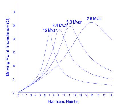
Figure 21. Variations in frequency response at 33 kV bus as a function of capacitor bank size
