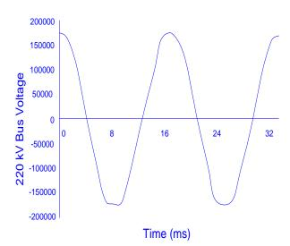
Figure 18. Line-to-neutral voltage at PCC
