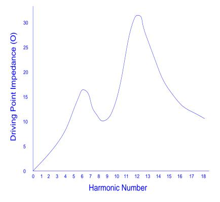
Figure 17. Driving point impedance at 6.6 kV bus7
